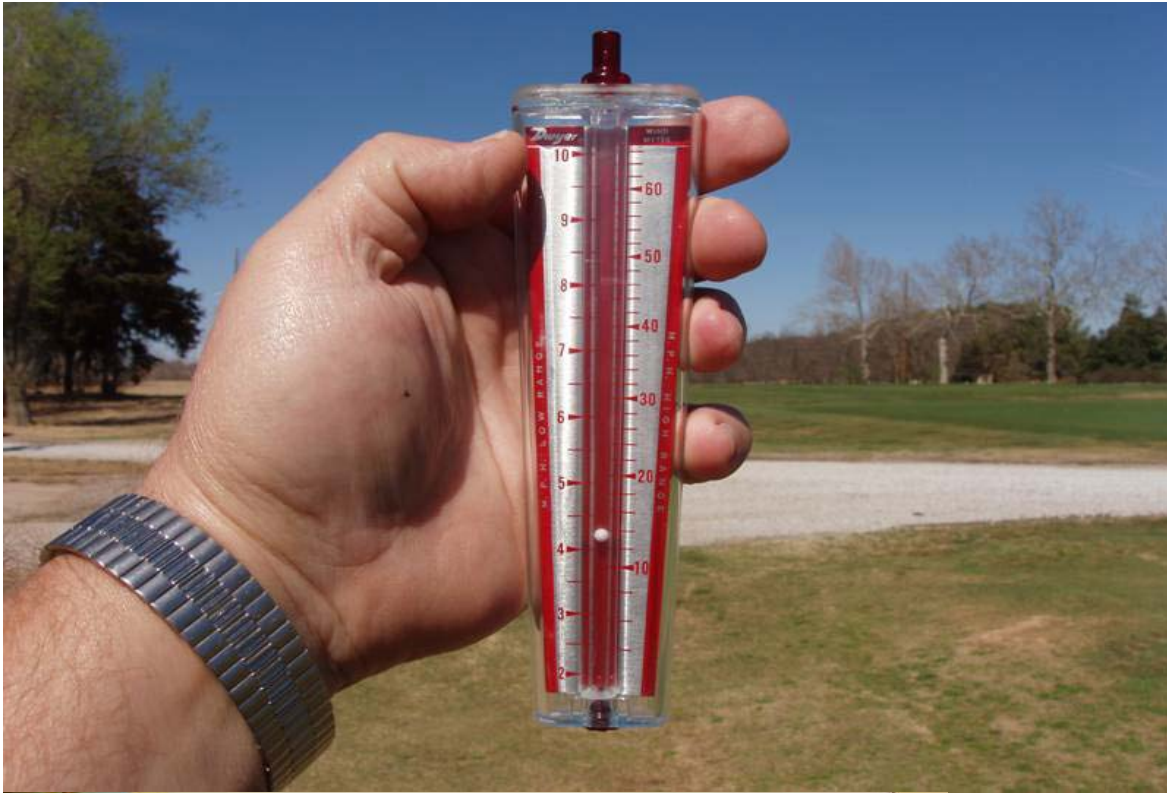
Figure 1. Dwyer Hand-held Wind Speed Meter Images.
