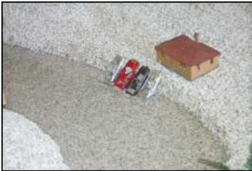
Arm the bank with junk cars. Note this does not protect the house for long.
