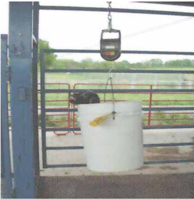
Figure 3-2. Fish scales and a plastic bucket make an excellent birth weight measuring system.
