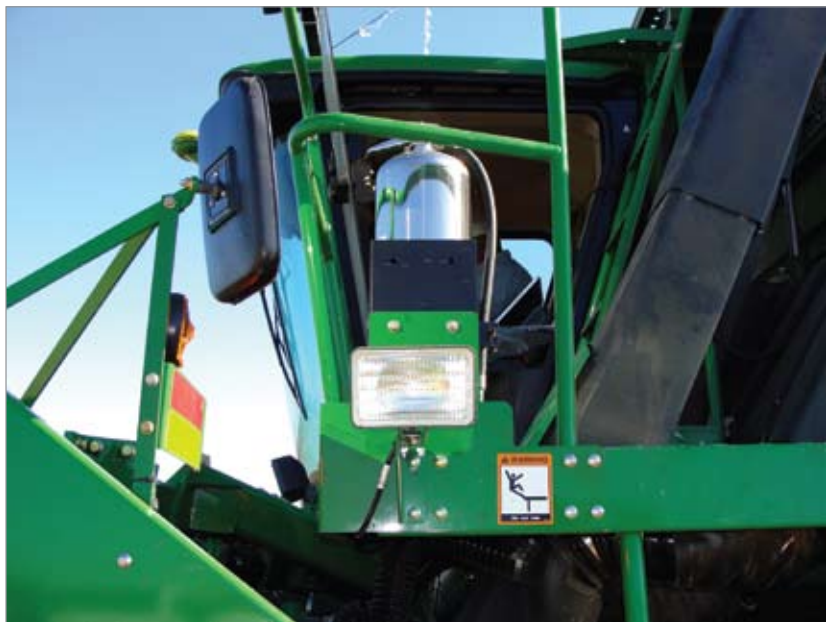
Platform water-based fire extinguisher.
