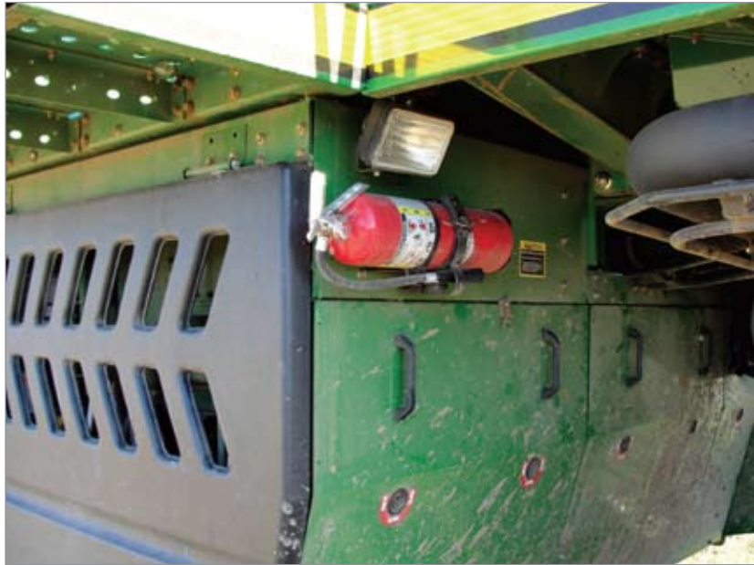
Engine compartment type ABC fire extinguisher.
