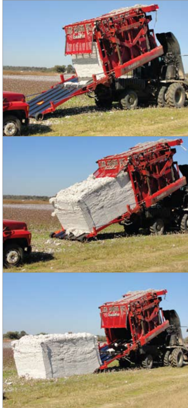
Case IH onboard module building picker unloading sequence.
