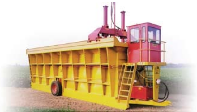
Figure 1 A modern module builder with cab for operator comfort and hydraulic drive system. A tractor provides PTO power to drive the hydraulic pump and drawbar power to move the builder. (Photo courtesy of KBH, Inc.)
