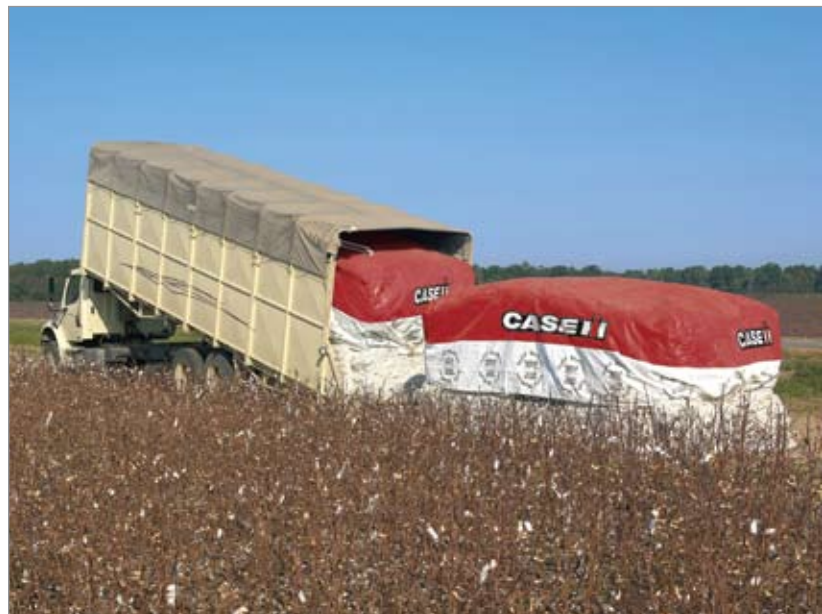
Figure 4 Two Case IH half-length modules staged together and being loaded into a module truck.
