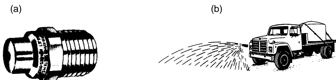
Figure 10.18. The (a) Solid-Stream Nozzle is Used for (b) Boomless Broadcast Herbicide Applications.
