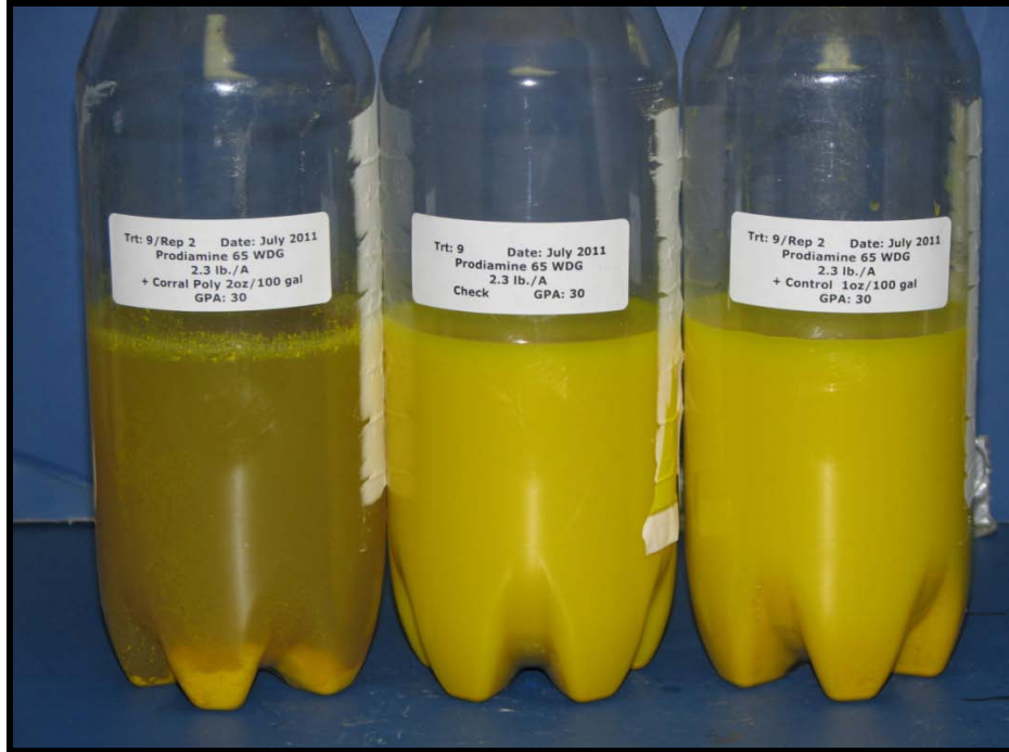
Figure 3. Incompatible mixture of Prodiamine 65 WDG and Corral® Poly (bottle on far left) and the compatible Control™ mixture in the far right bottle. Bottle in the middle is a controlled check with only Prodiamine 65 WDG.
