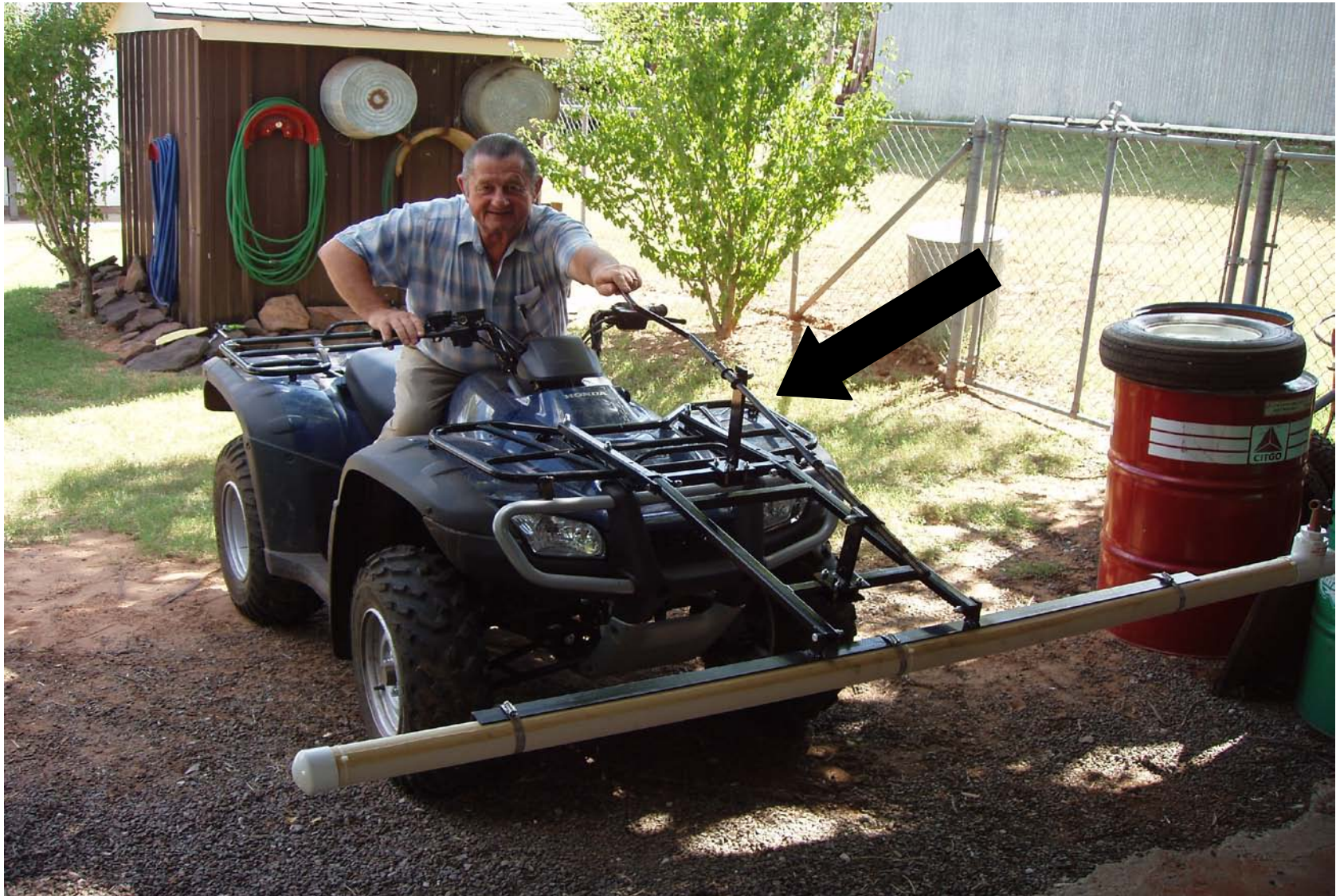
Figure 1. Image of ACR Sales ATV/Utility Vehicle Bracket Mounted to Honda 4-Wheeler.
