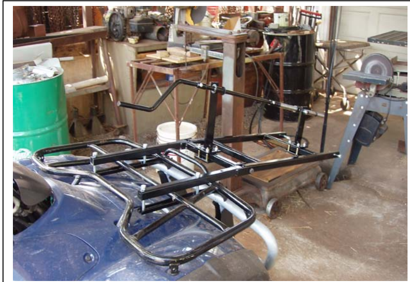
Figure 4. Images of ACR Sales ATV/Utility vehicle bracket and Speidel Wiper boom mounting on ATV.
