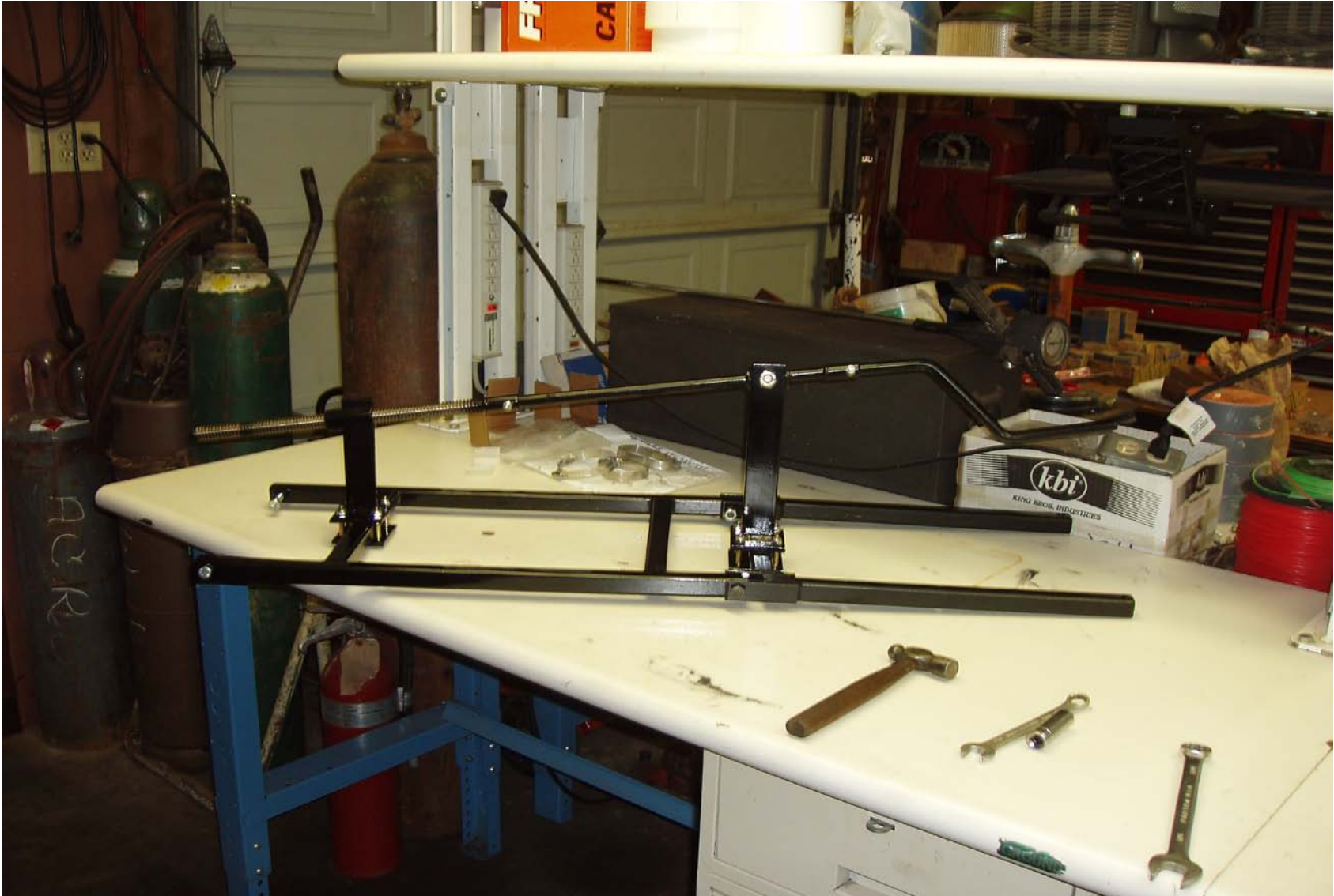
Figure 2. Image of ACR Sales ATV/Utility Vehicle Bracket Assembled Prior to Vehicle Mounting.
