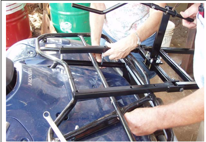
Figure 4. Images of ACR Sales ATV/Utility vehicle bracket and Speidel Wiper boom mounting on ATV.
