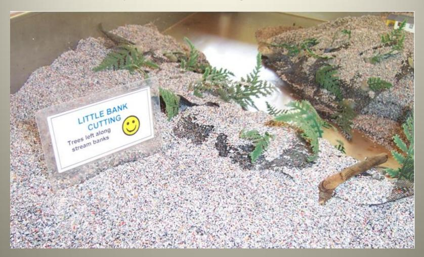
We simulate riparian vegetation using plastic foliage attached to window screen. Typically we will install "vegetation" on one meander, leave another meander unvegetated and then observe the difference in stream bank erosion, channel widening, and fish habitat in the form of scour holes, shade and depth for cooler water etc.
