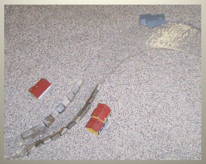
If you have a problem situation, the stream trailer may be able to duplicate what is happening or can happen. Here we see how upstream bank armoring leads to downstream flooding and property damage.
