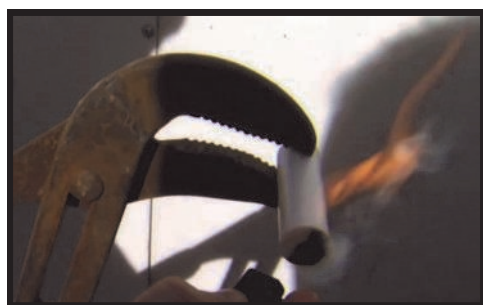
A smoke emitter used to conduct a smoke test.
