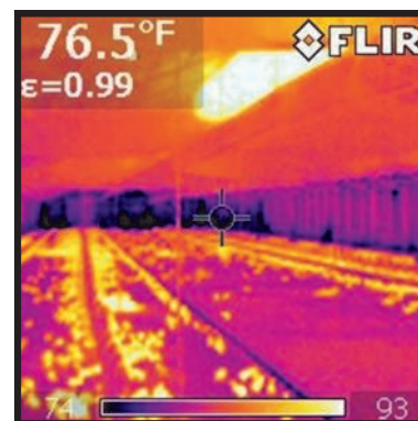
Thermal imagery of the inside of a broiler house. Colder areas are shown as purple and hotter areas are shown as orange.
