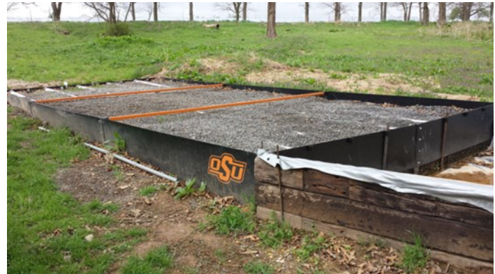
Phosphorus drainage filter installed at a poultry farm.
