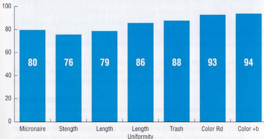
*Results were obtained with permitted tolerances of: Length, 0.02 inches; Length Uniformity, 1.0 percent; Strength, 1.5 g/tex; Micronaire, 0.1 units; Color Rd, 1.0 units; Color +b, 0.5 units; Trash, 0.1 percent area.*
