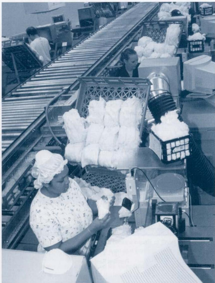
*Utilizing the latest technology and equipment, samples are classed on an assembly-line arrangement with fiber measurement results electronically transmitted to the classing facility's computerized data base.*
