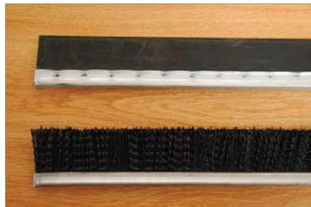
Close-up image of a new bat (top) and brush (bottom) used on stripper rolls.
