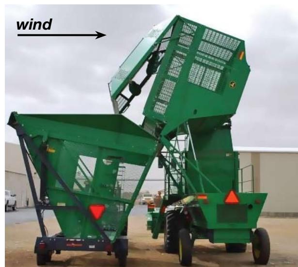
Cotton stripper unloading into a boll buggy shown with basket rotating into the wind.
