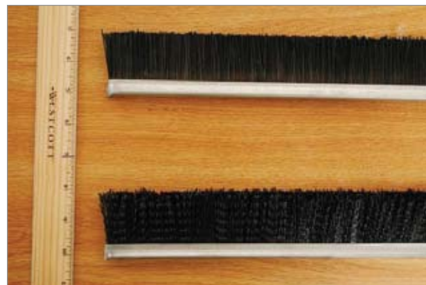
Image of brush-bat (uncrimped nylon bristle brush, top) and conventional brush (bottom).
