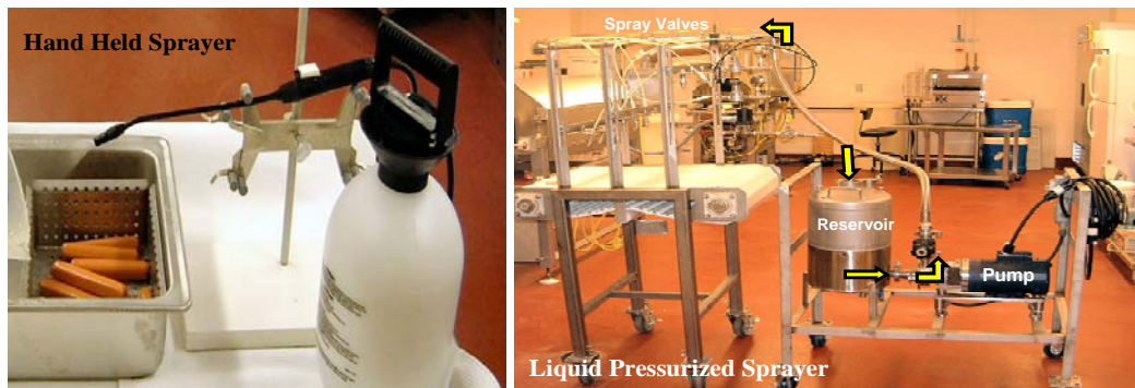
Figure 1. Equipment used for spraying electrolyzed water onto meat products. Handheld manual sprayer (left) and automated pressurized sprayer (right).
