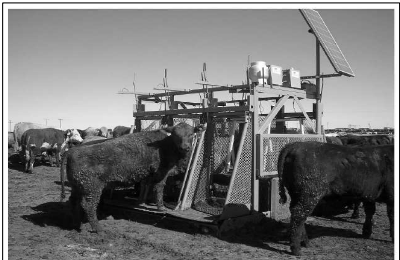
Figure 1. The GrowSafe Beef in-pen weighing equipment (GrowSafe Systems, Ltd.). Source: Kolath et al., 2007
