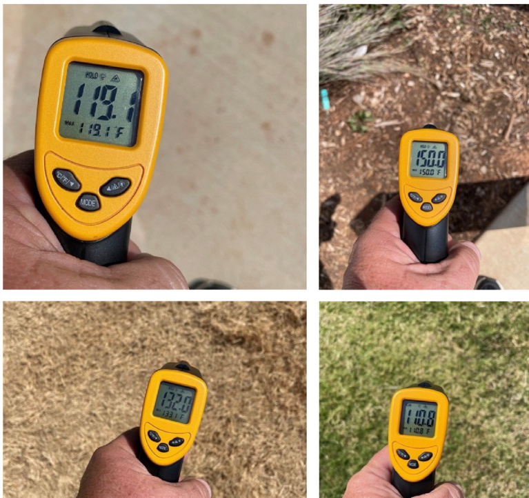
Figure 66: An infrared thermometer taking the temperature of concrete, brown wood mulch, dead grass and living grass (Shelley Mitchell).
