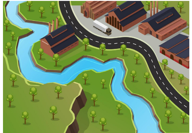
Figure 85: Rivers flow faster on the outside of curves. This river will eventually take out the street in two places.
