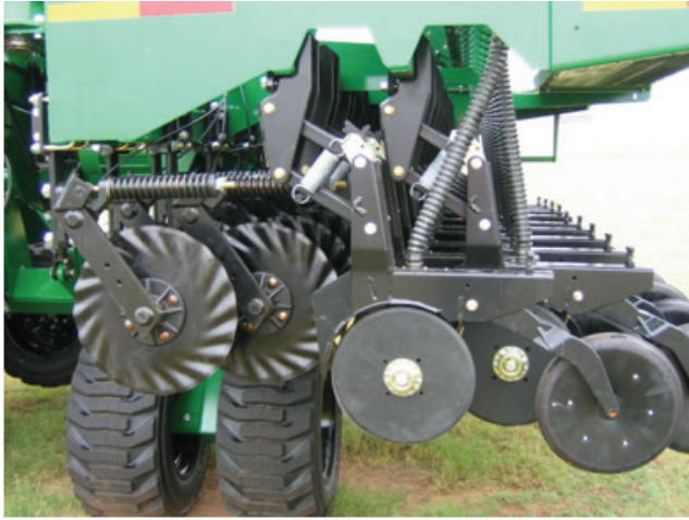
Figure 1. Some no-till drills use a coulter that slices through residue and performs a small amount of tillage in front of the disc-opener.
