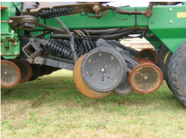
Figure 2. One of the most popular no-till drill designs uses a single disc opener that slices through residue and opens the seed trench.
