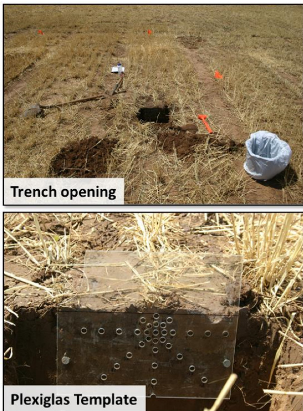
Figure 1. Upper photo illustrates the trench opening procedure adopted in field, perpendicular to wheat rows, with the objective to evaluate the pH distribution in the soil profile. Bottom photo shows a plexiglass template used to ensure all pH measurements were taken centered at the furrow and at constant distances from the original pelletized lime application placement.
