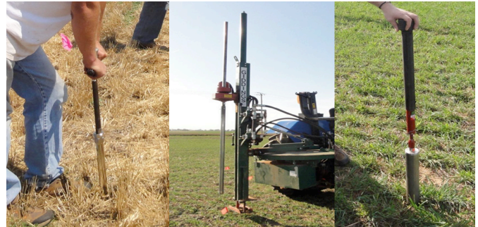
Figure 1. From left to right, Push Probe (diameter 2.26 cm), Giddings Probe (diameter 3.96 cm), and slide hammer soil sampling probe (diameter 4.8 cm).
