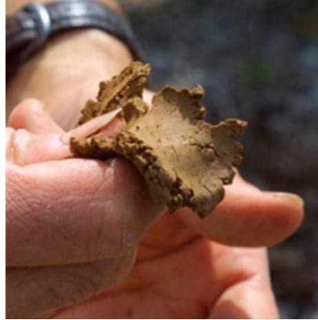
Figure 7. Soil quality matters immensely. The ribbon test is a quick, on-site test for adequate clay content. Not all high clay content soils are suitable for dams - ideally a mixture of clay, sand and silt is needed to allow for good compaction.
