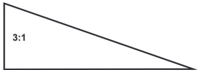
Figure 11. A generally advantageous slope for dam faces and shorelines is 3 feet of “run” for every 1 foot of “rise” (3:1). This reduces erosion potential, decreases the chances of child drownings and makes it possible to mow dam faces to eliminate young trees. Image courtesy Alabama Cooperative Extension Service.
