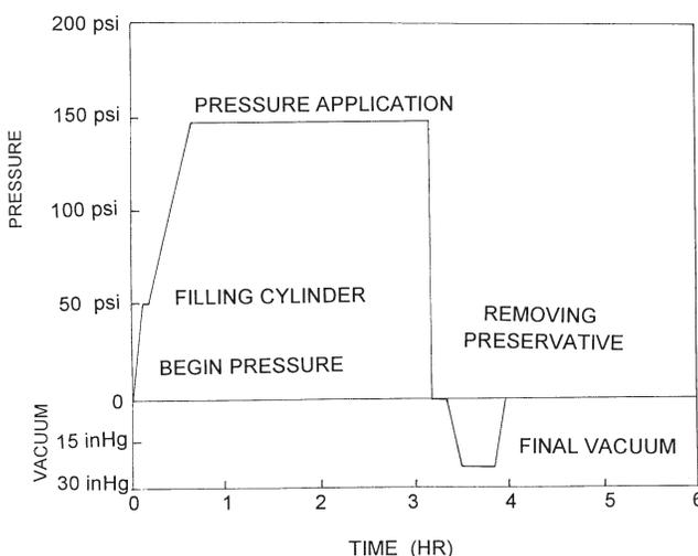
**Figure 6. A typical empty-cell treatment schedule.**
