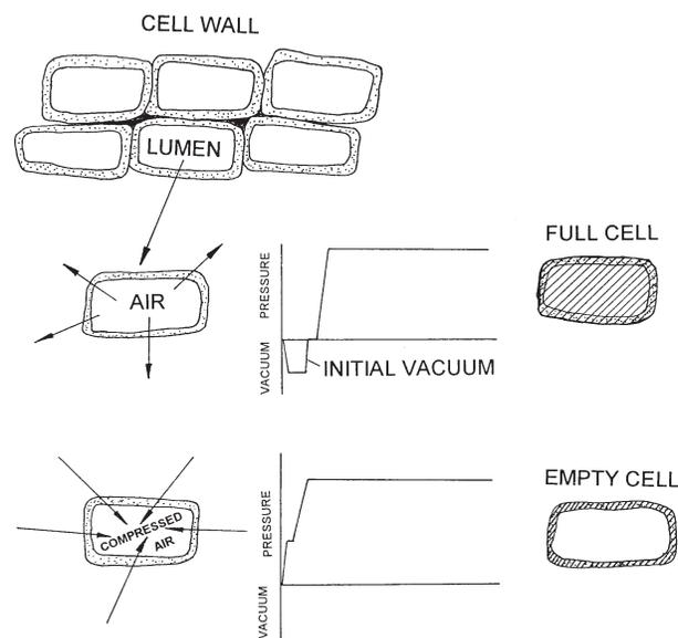
**Figure 4. Schematics illustration between full-cell and empty-cell treatment methods.**
