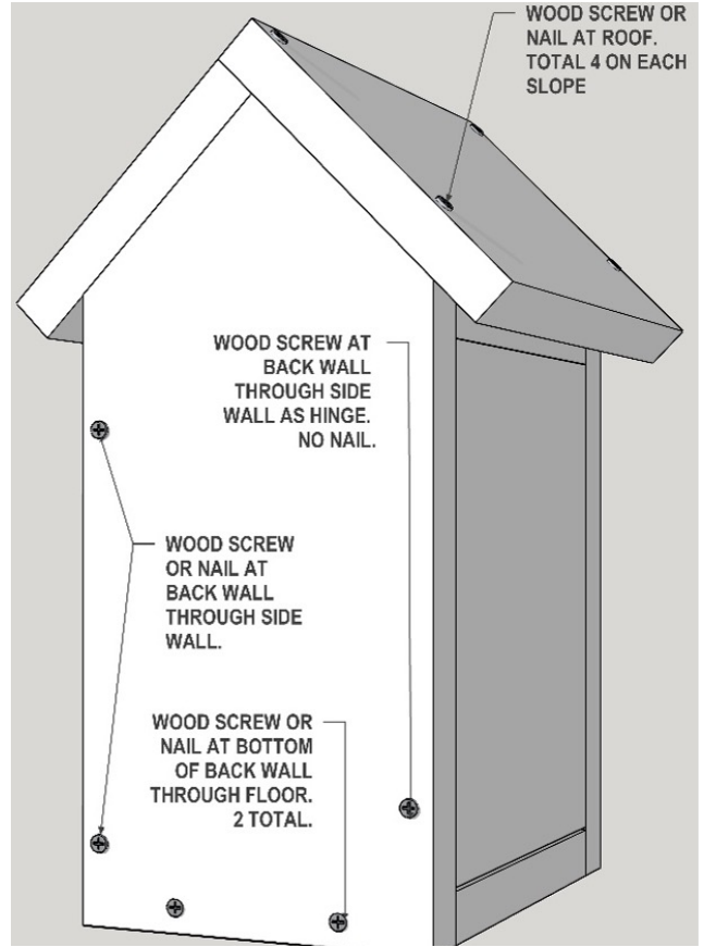
Diagram B7. Screw and nail positions at the back
