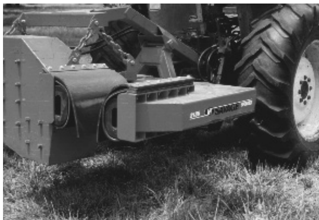
Figure 2. A Pecan Shaker Equipped with Donut Pads.
