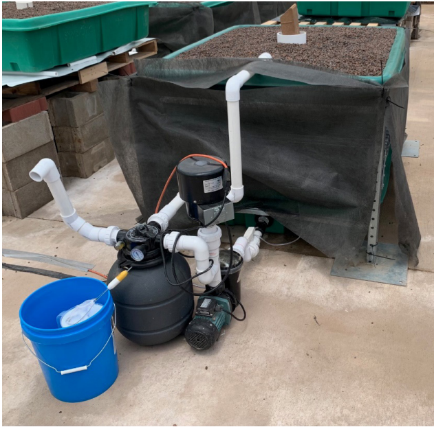
Figure 4. Small-scale 20 square feet media bed aquaponics system, donated by Symbiotic Aquaponic LLC. The filtration system in the center is an Aquadyne mechanical bead filtration unit. (Image Credit: Che Deer-Graduate Student at Oklahoma State University).
