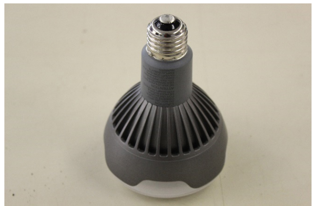
Figure 1. Heat sink and standard E26 light bulb base fitting of Philips® GreenPower LED flowering lamp.
