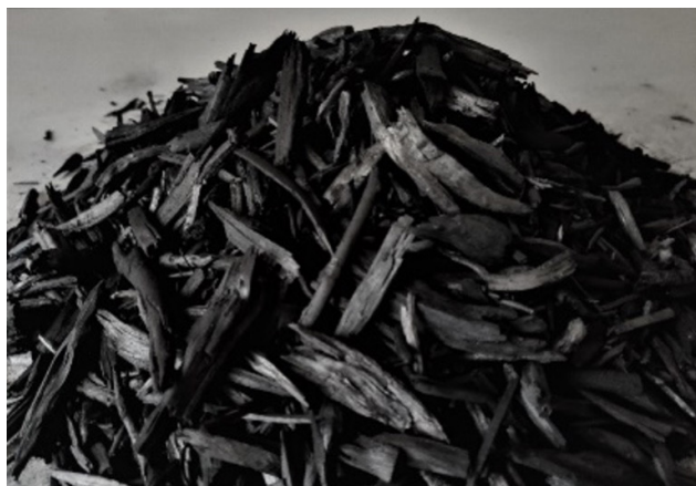
Figure 2: Eastern red cedar mulch biochar prepared from double barrel system.
