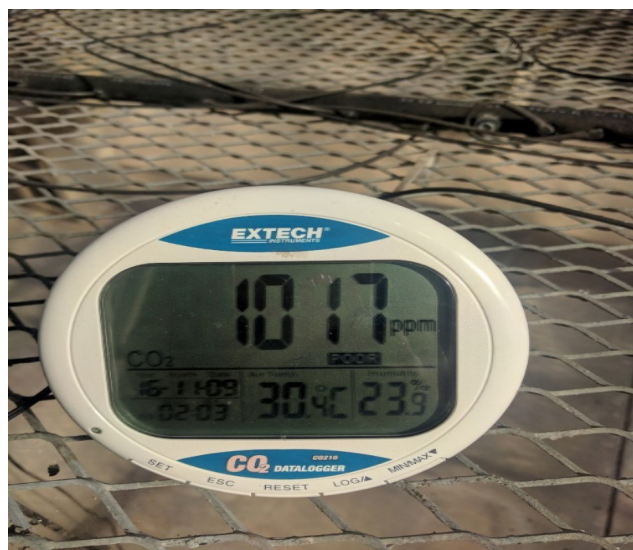
Figure 6. Extech CO 2 Monitor (FLIR Commercial Systems Inc., Nashua, NH) and data logger. It measures CO 2 , temperature and humidity and has 15,000 data log storage capacity.
