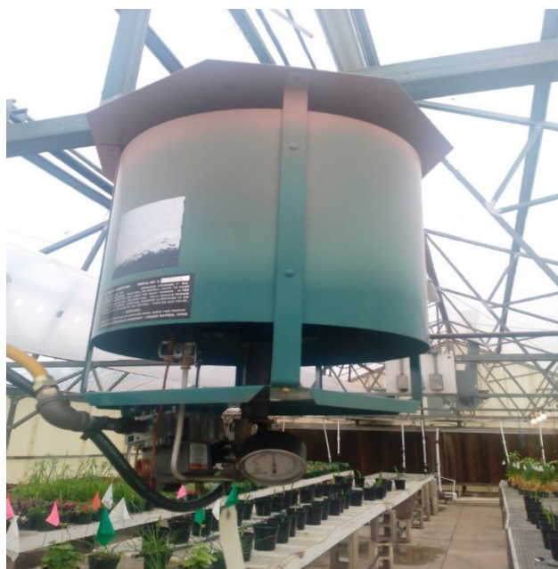
Figure 3. Carbon dioxide generator manufactured by Johnson Gas Appliance Company (Iowa). The generator operates with either propane or natural gas and has pressure gauge to control the size of burner.
