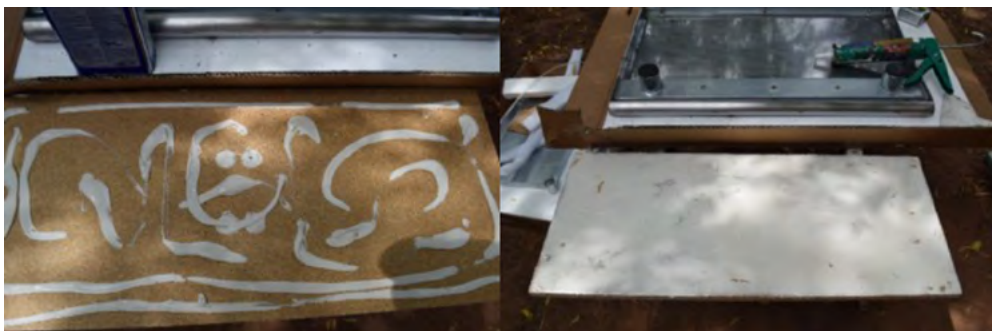
Figure 7. Adhesive spread on MDF sandwich board. Left shows globs of adhesive, and right photo shows the adhesive spread into a film. Note that the screw heads and washers for mounting the vibration motor were completely covered with adhesive
