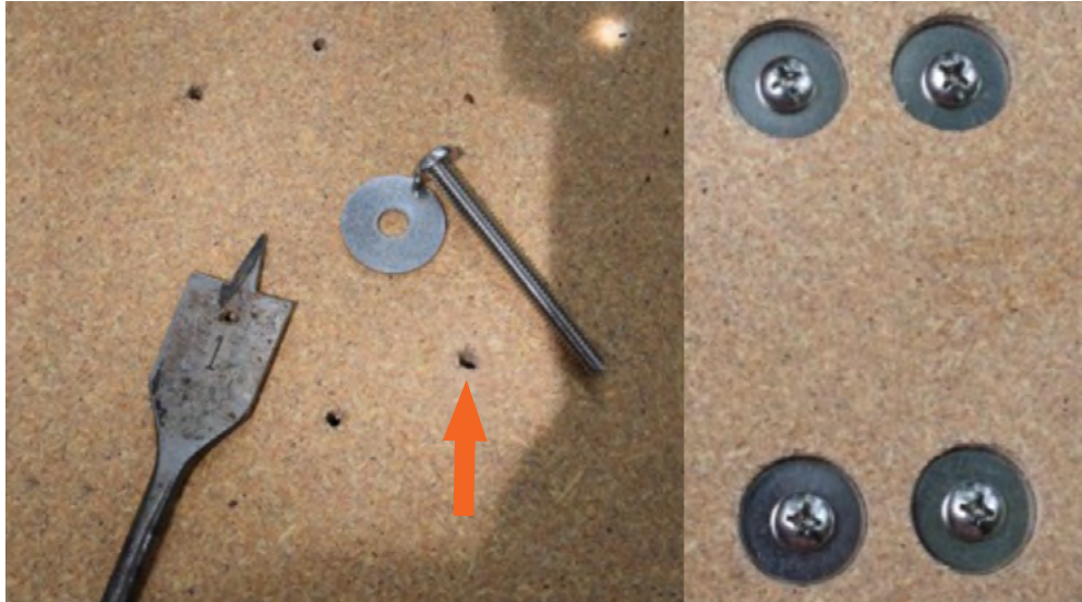
Figure 6. This figure shows two photos of the face of the MDF sandwich board that will be glued to the underside of the tabletop. The photo on the left includes a 1" spade drill bit that was used to countersink the MDF surface at each pilot hole for the vibration motor mount screws (orange arrow indicates one of the four pilot holes) to recess the washers and screw heads. Photo on the right shows the washers and screws inserted into the board after countersinking and drilling the pilot holes to full size. [Note: countersink the pilot holes before drilling holes to full size to prevent centering issues with the spade bit.]
