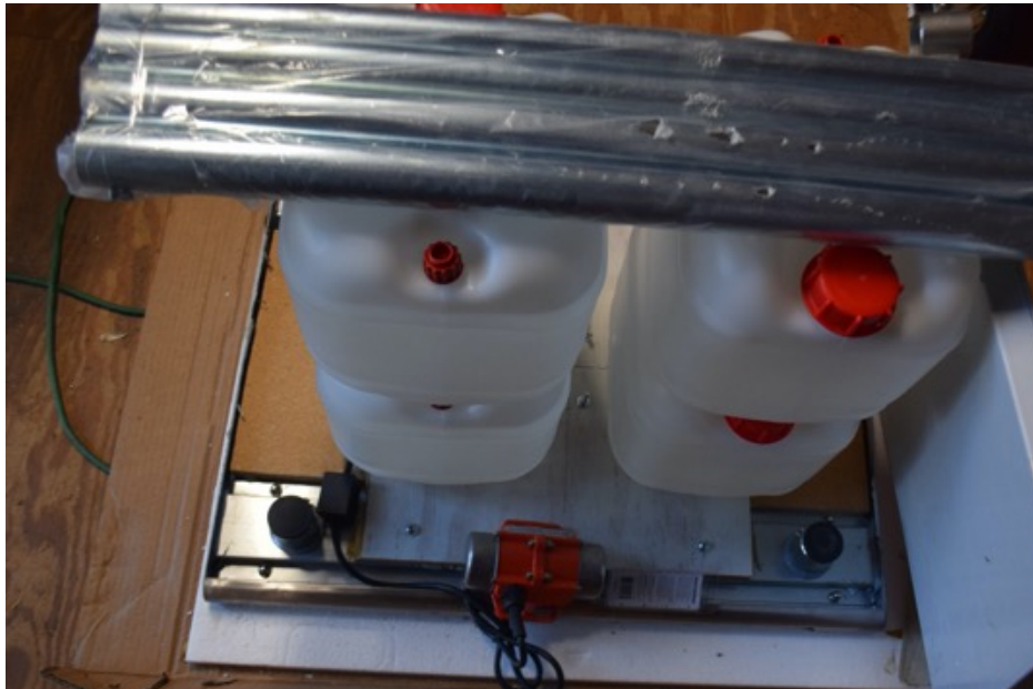
Figure 10. Weights (water-filled containers and table legs) were stacked on the plywood support board to help promote glue and surface contact. Water mass was about 44 kg.
