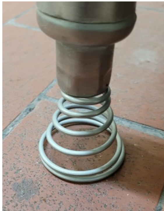
Figure 12. Conical spring supporting table leg. In this example, the spring is fixed to the bottom of the table leg and has not been secured to the floor.
