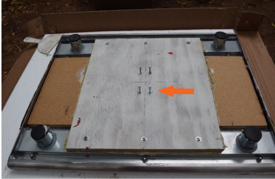
Figure 9. Plywood support board glued and screwed to the underside of the tabletop and the MDF sandwich board. Note the four mounting screws for the vibration motor (one screw indicated by an orange arrow), tightened in place with temporary nuts and washers.
