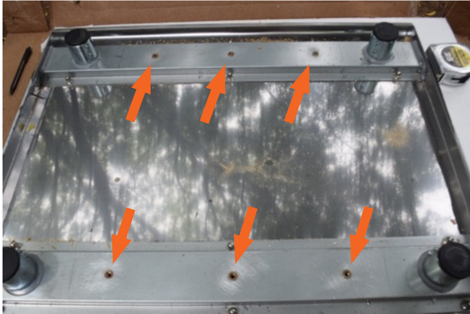
Figure 4. Shows placement of six, 1/4-20 rivnuts in the support channels of the underside of the table. The rivnuts were used to mount the support board.
