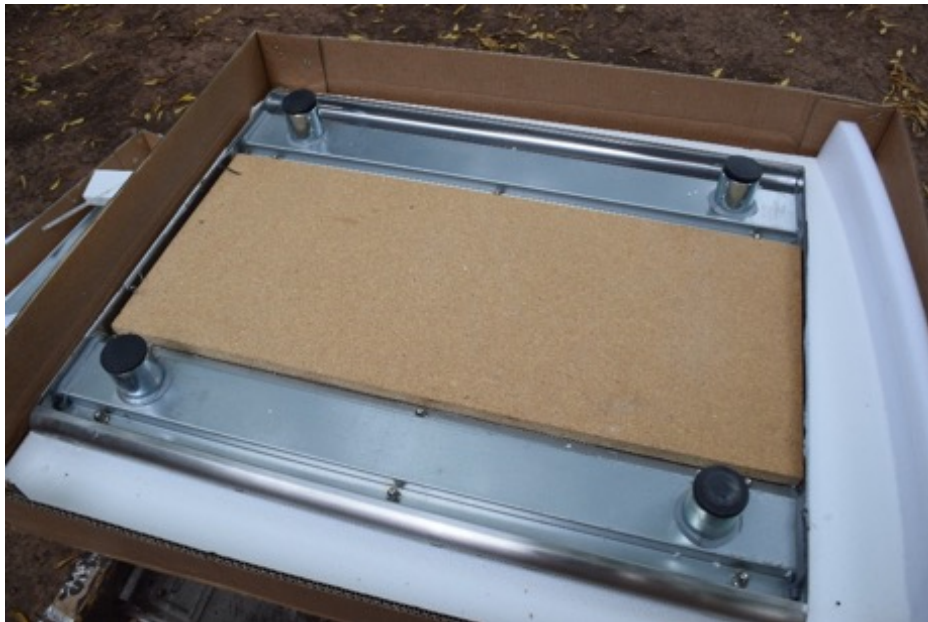
Figure 2. Underside of stainless steel tabletop, showing the two support channels and the MDF sandwich board that was cut to fit between the channels.
