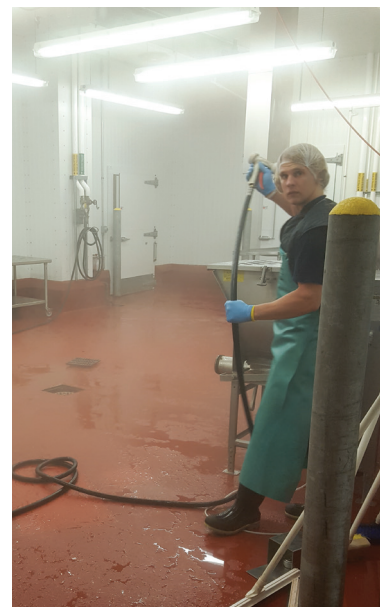
Figure 1. Condensation occurring during a cleaning process in a refrigerated room of a meat-processing facility.
