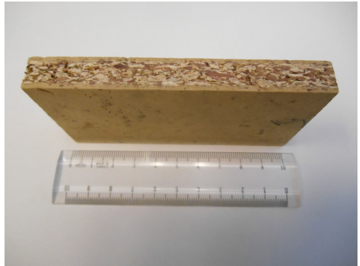
Figure 1. Cross section of sandwich type panel.
