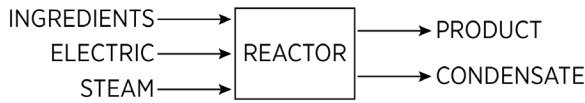
(a) Initial process element shows a basic reactor vessel for an enzymatic reaction.
