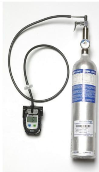
**Figure 10. Bump test kit.**
