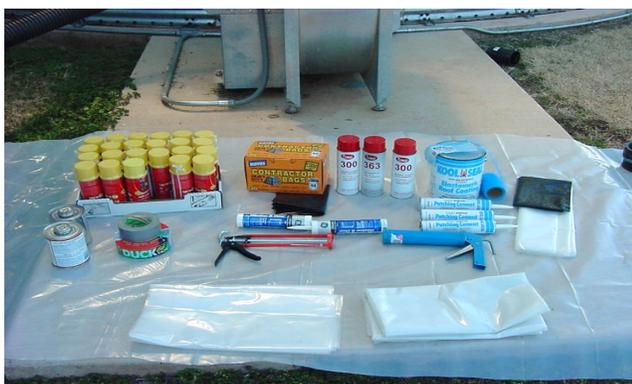
**Figure 3. Products used for sealing grain structures.**
