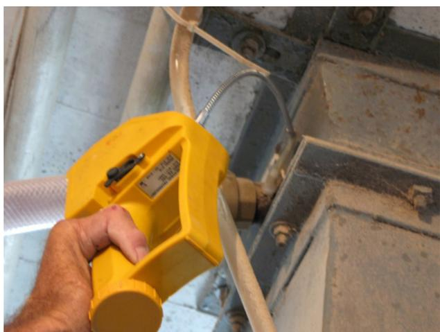
**Figure 9. Using an electronic gas detection monitor to determine the level of phosphine gas.** (Photo: Edmond Bonjour)
