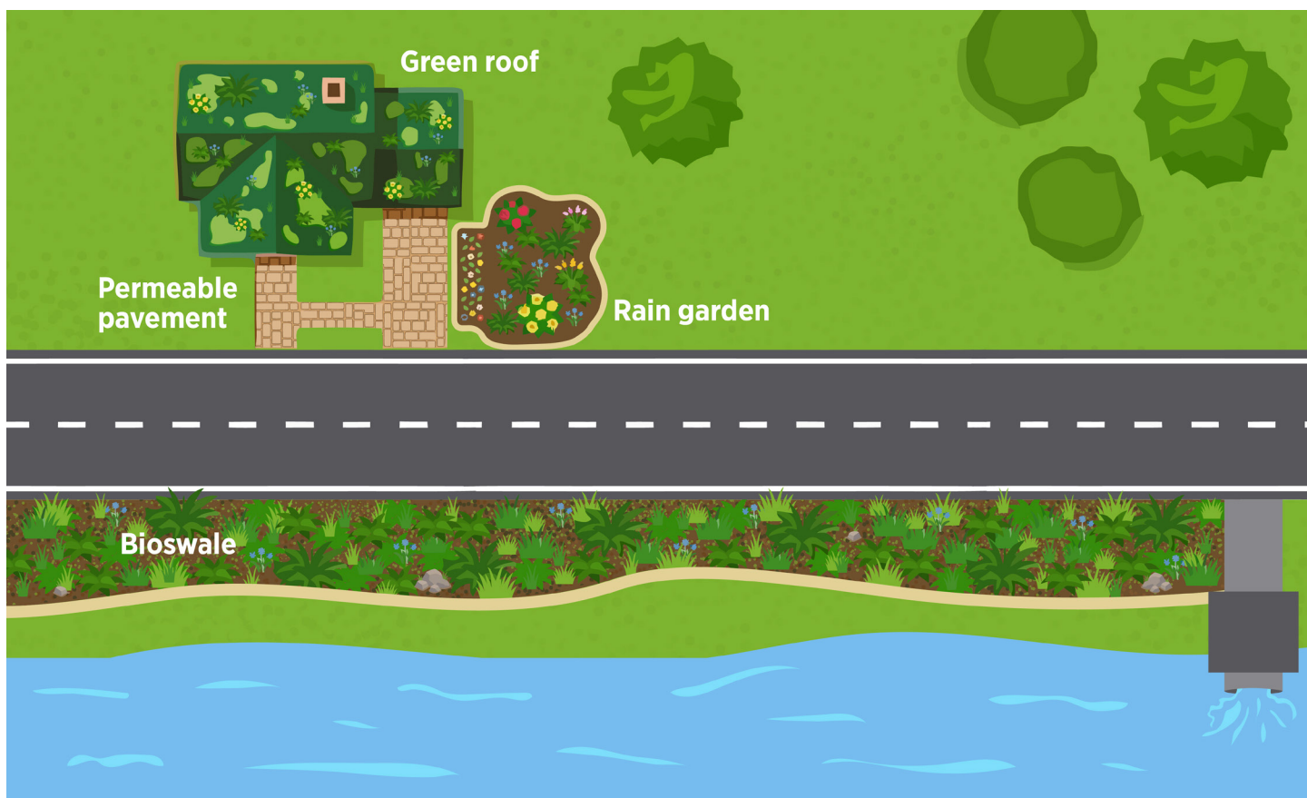
Figure 3. Green infrastructure practices used for runoff reduction and control. Green roof: Vegetation on rooftops reduces runoff and improves insulation. Permeable pavement: Allows water to infiltrate through the surface. Rain garden: Depressed landscaped area that captures and filters runoff. Bioswale: Vegetated channel that slows runoff, filters pollutants and promotes infiltration.
