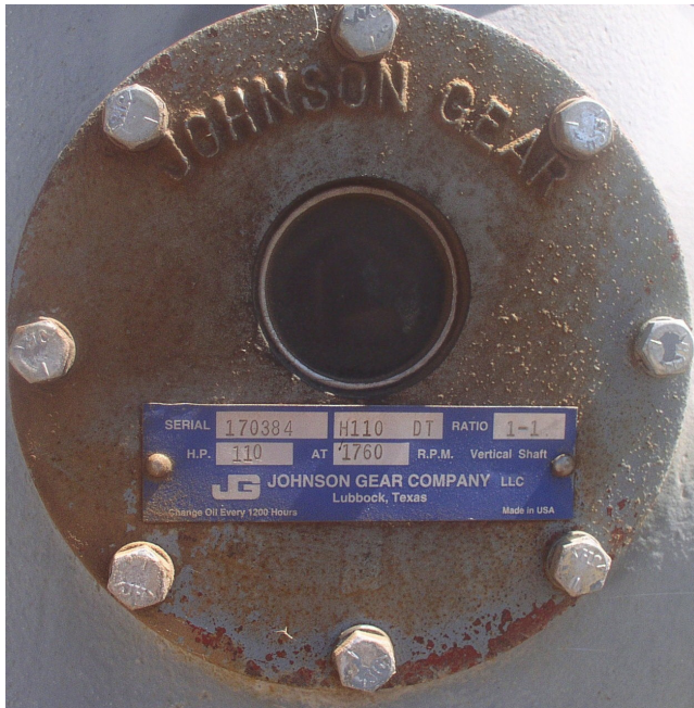
Figure 6. Gear Drive nameplate for a 1:1 (non-reduction) drive ratio.
