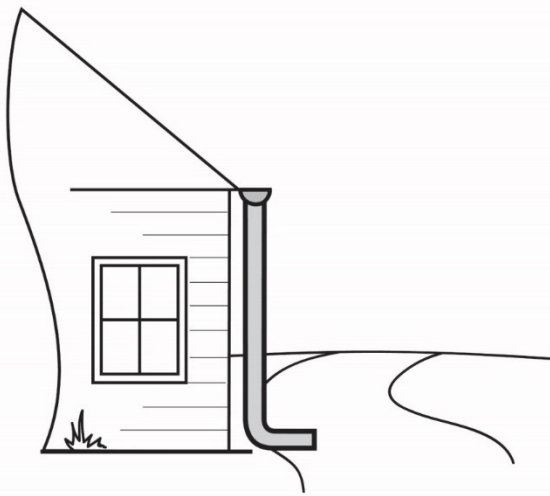
Figure 3. Downspout discharges on driveway.
