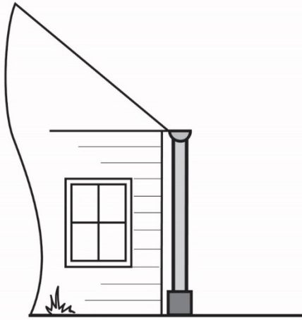
Figure 2. Downspout connected under the ground surface.
