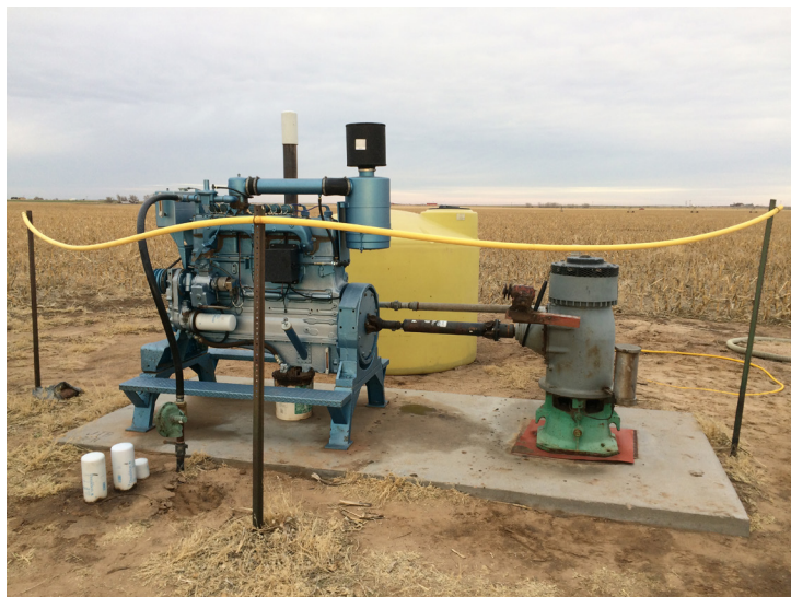
Figure 3. A natural gas engine extracts groundwater for irrigation.
