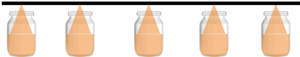
Figure 6. Place a container under each nozzle to see if all jars fill in about the same time.
